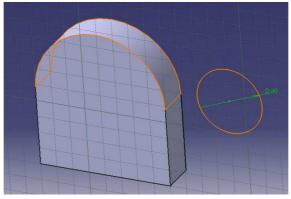
Use **Constraints Defined in Dialog Box** to create *Concentricity* constraint. The circle should be moved to the center of the arc automatically.
