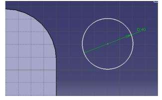
Next, locate the center of the circle in the same point as the center of the arc. The *Concentricity Constraint* must be created.
