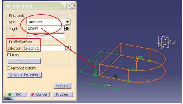
Using **First Limit Type** option as <u>Dimension</u> user can define the height of the created 3D model. Use **Preview** button to see the result. **OK** button allow to accept results.
